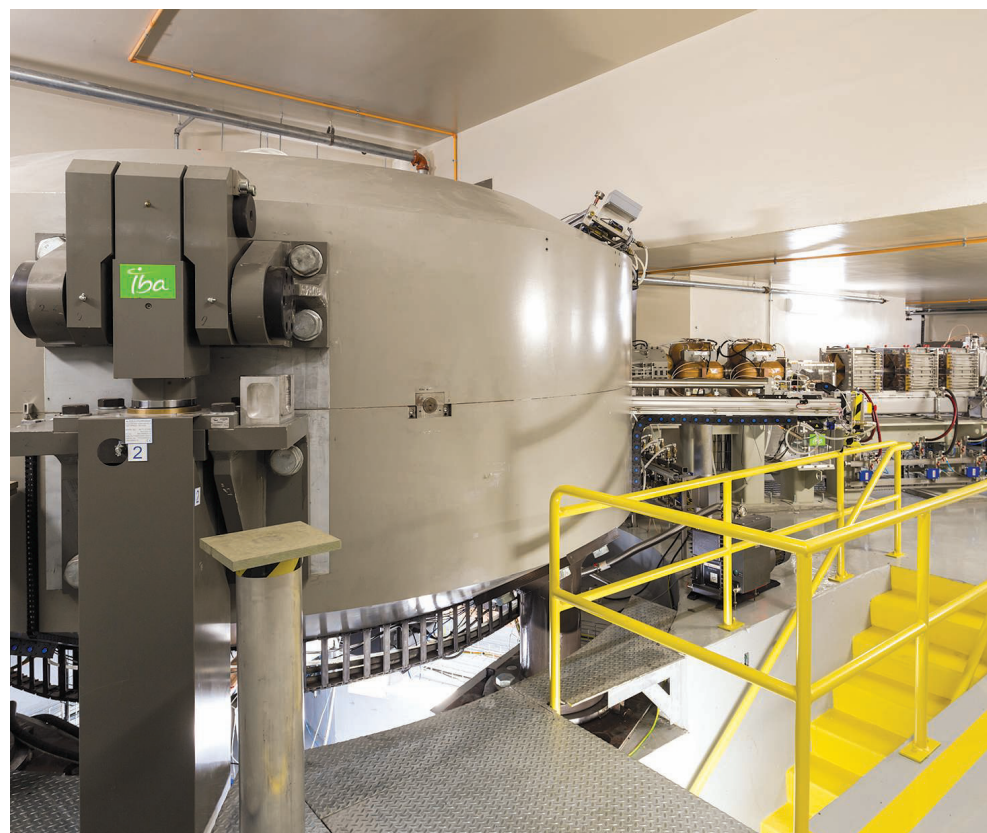
The 220-ton cyclotron accelerates protons and sends them down the beamline.
