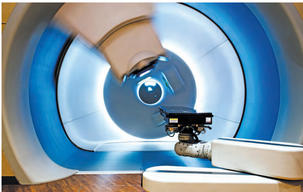
Texas Center for Proton Therapy's "Hope" treatment room includes an isocentric gantry, which rotates the proton beam angle 360 degrees around the patient.
