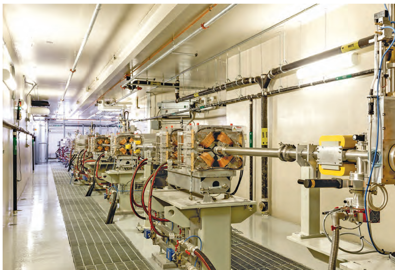
Protons generated by a cyclotron travel down a beamline at almost the speed of light.
